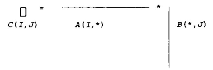
In IJK, matrix C is calculated in a row by row fashion where each row is obtained from a sequence of inner products of one row of A with all columns of B. JIK generates C column by column from a sequences of inner products of all rows of A with one column of B.
