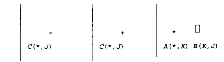
In KJI, all columns of C are updated by a column of A scaled by the elements of one row of B. In JKI, a column of C is calculated at a time by accumulating in it columns of A scaled by elements of a column of B.
