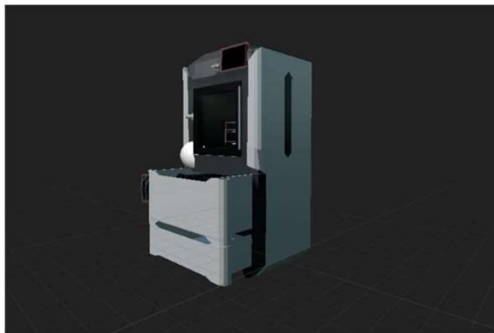
Figure 2. 3D model of Stratasys F170 3D printer in Unreal Engine 4.
