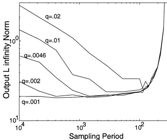
Fig. 7. Lower bounds on  $L^\infty$  performance as a function of sampling rate and quantizer precision.
