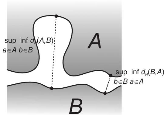
Figure 3: Illustration of the Hausdorff distance between sets A and B:
