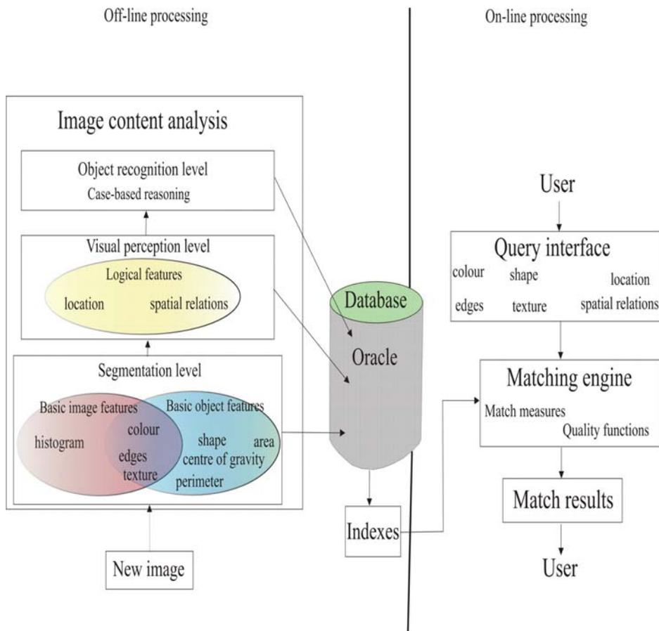
Figure 2: Block diagram of our content-based image retrieval system
