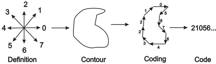
Figure 6: Chain code representation based on the 8-connectivity
