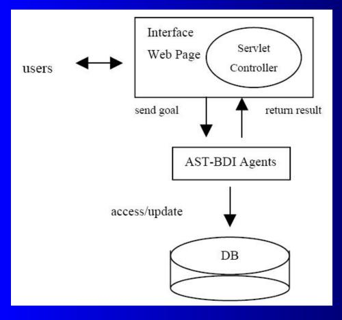
The whole system consists three parts: •The first level is the Servlet Controller, which is a link between users and BDI agents. It provides user interface and dynamically generates corresponding web pages.
