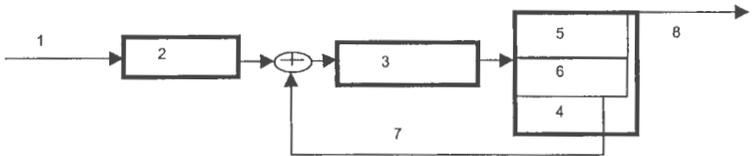
**Fig. 1** Diagram of the investigated wastewater plant: 1 – wastewater inflow; 2 – primary clarifiers; 3 – aeration basins; 4 – secondary clarifiers; 5 – purification zone; 6 – sedimentation zone; 7 - extern recirculation; 8 – outlet of the purified wastewater
