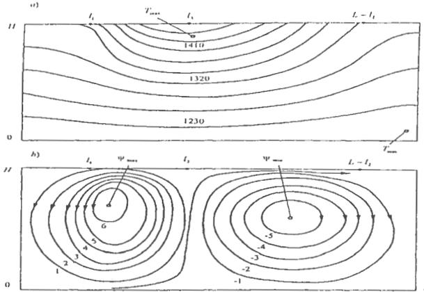
**Figure 2.** Computed temperature (figure a) and current distribution (figure b) in the glass melt for the longitudinal section of the glass tank furnace.
