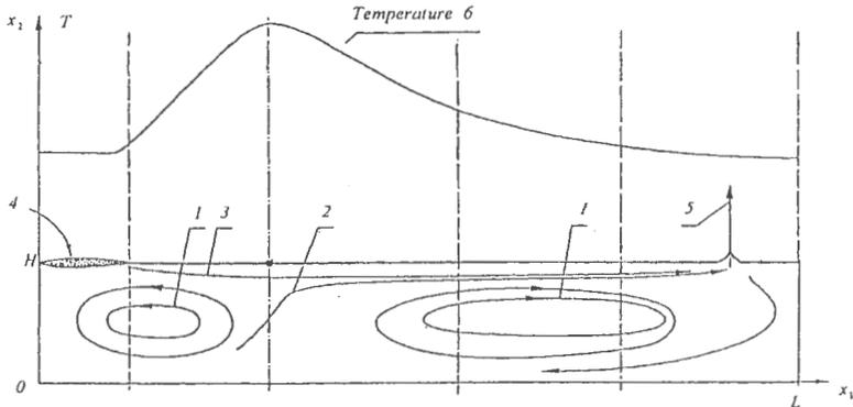
**Figure 1.** Longitudinal section of the glass tank furnace and the main currents occurring in the melt; 1,2,3 - rotating, withdrawal and surface current, respectively, 4 - raw materials input, 5 - glass take-out, 6 - temperature distribution on the free surface of the glass melt.
